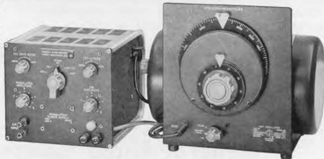
Figure 3. The Type 1264-A Modulating Power Supply is shown (above) relay-rack mounted with the Type 1361-A UHF Oscillator and (below) used on a laboratory bench with the Type 1218-A Unit Oscillator.
